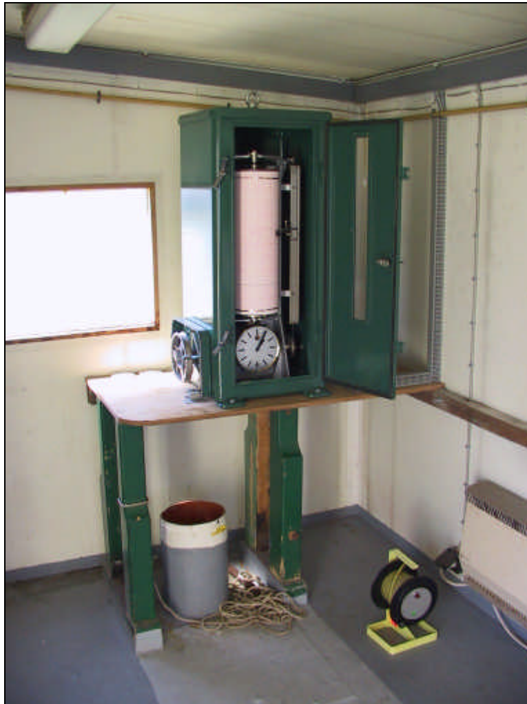
In the monitoring station in Oostende, which is located at the entrance of the Montgomery Dock, a maregraph is used to monitor the relative sea level by registration of the height of a float in the damping tank. The damping tank ensures that the water levels can be monitored without too much interference from waves or passing ships. The registered water level is regularly checked with a tape measure emitting a sound signal upon contact with water (Flemish Hydrography).
